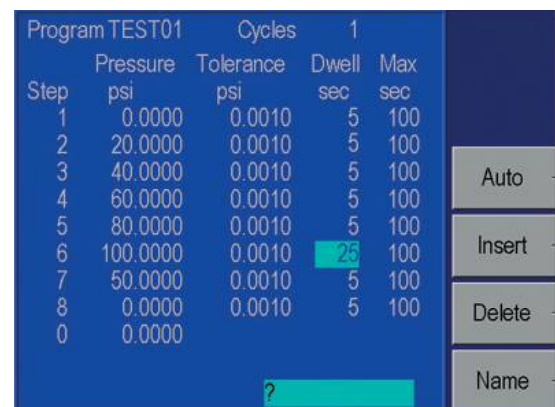
All Series 7250s are fully programmable and can store up to 20 separate programs with up to 1000 steps.
