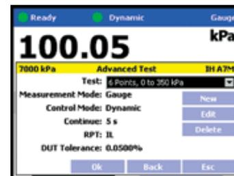
PPC4 supports setting up and running quick tests on the fly and creating and storing complex test sequences for recall and execution.
