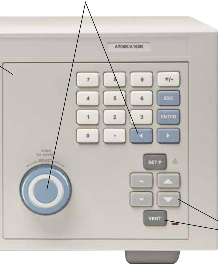
Direct pressure control keys for simple setting, venting and slewing or jogging of pressure
