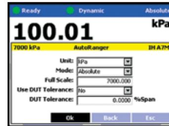
PPC4's AutoRange feature optimizes measurement, control and safety features for the specific range of the test being run with a few simple entries.
