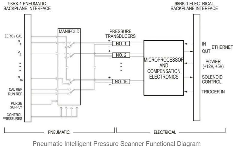
Pneumatic Intelligent Pressure Scanner Functional Diagram
