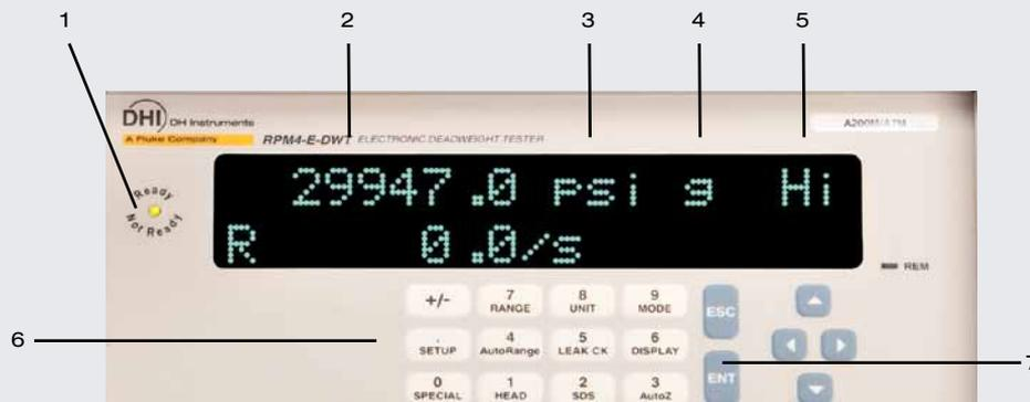
1. Pressure "Ready" (green) "Not Ready" (red) based on real time measurement of pressure stability
