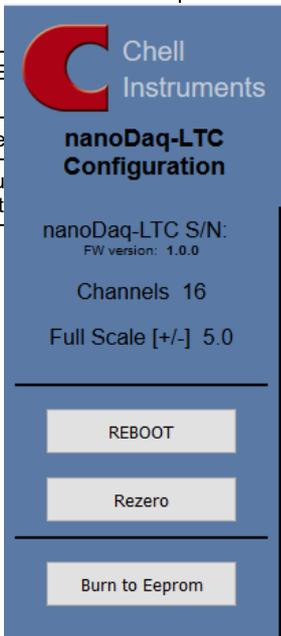
The sidebar is a blue vertical panel on the left side of the webserver interface. At the top is the Chell Instruments logo. Below it, the text reads 'nanoDAQ-LTC Configuration'. Further down, it displays 'nanoDAQ-LTC S/N:' followed by 'FW version: 1.0.0'. Below that, it shows 'Channels 16' and 'Full Scale [+/-] 5.0'. At the bottom of the sidebar, there are three buttons: 'REBOOT', 'Rezero', and 'Burn to Eeprom', each in a light grey box with black text.
